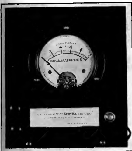
Front view of output meter.
